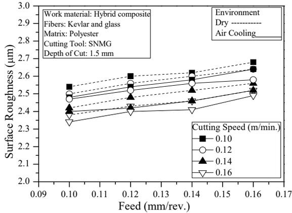
**Fig. 2.9** Variation of  $R_a$  with  $S_o$  at different  $V_c$  and 1.5 mm depth of cut under both dry and CAC condition
