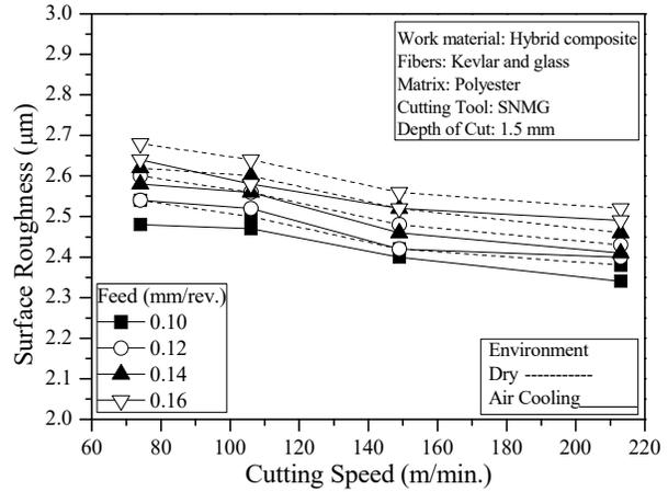
**Fig. 2.12** Variation of  $R_a$  with  $V_c$  at different  $S_o$  and 1.5 mm depth of cut under both dry and CAC condition
