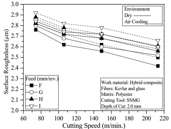
**Fig. 2.13** Variation of  $R_a$  with  $V_c$  at different  $S_o$  and 2.0 mm depth of cut under both dry and CAC condition
