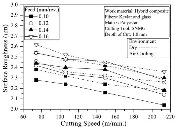
**Fig. 2.11** Variation of  $R_a$  with  $V_c$  at different  $S_o$  and 1.0 mm depth of cut under both dry and CAC condition
