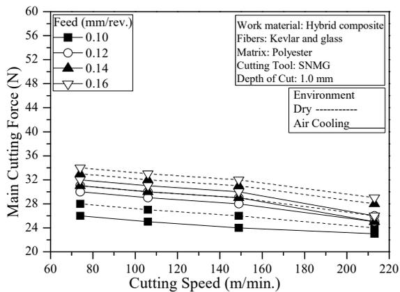
**Fig. 2.5** Variation of  $P_z$  with  $V_c$  at different  $S_o$  and 1.0 mm depth of cut under both dry and CAC condition
