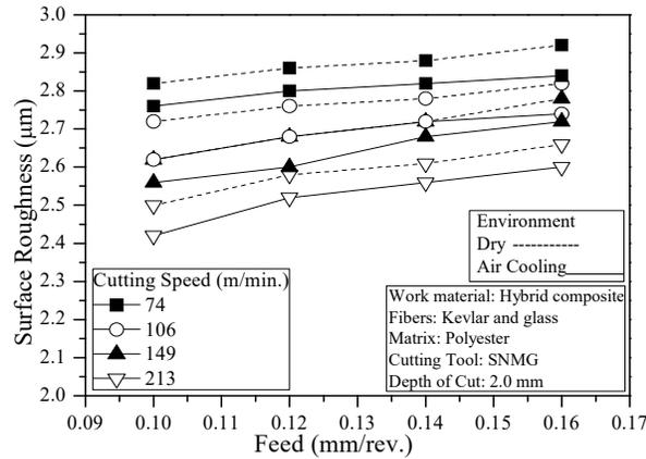
**Fig. 2.10** Variation of  $R_a$  with  $S_o$  at different  $V_c$  and 2.0 mm depth of cut under both dry and CAC condition
