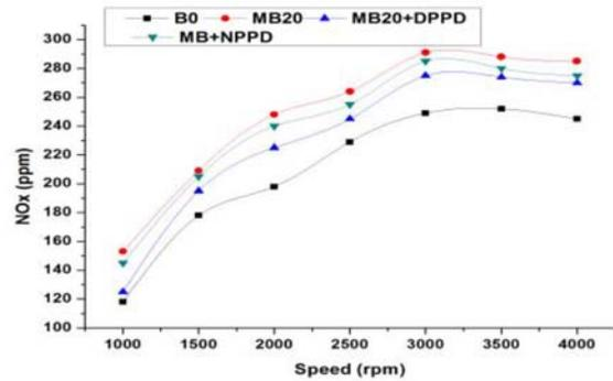
**Fig 2:** Fluctuation of NOx emission at different speed
