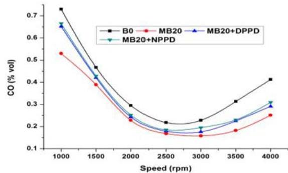
**Fig 3:** Fluctuation of CO emission at different speed
