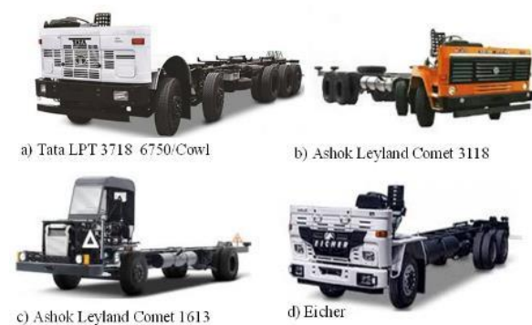
Figure 4: Cowl and chassis (incomplete truck body), adapted from [23-25]
