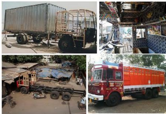
Figure 10: Road side truck body and cab building in India
