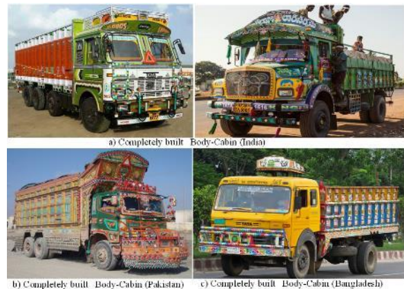
Figure 3: Road side builders-made complete truck body-cabins in South Asia, adapted from [12]
