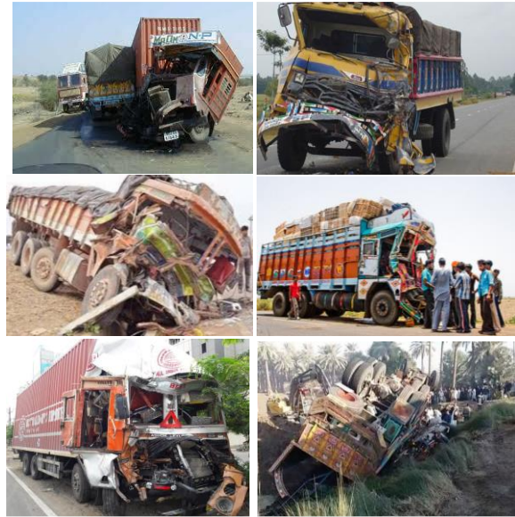
Figure 11: Crashed truck cabins have no means to absorb impact (India, Bangladesh & Pakistan)
