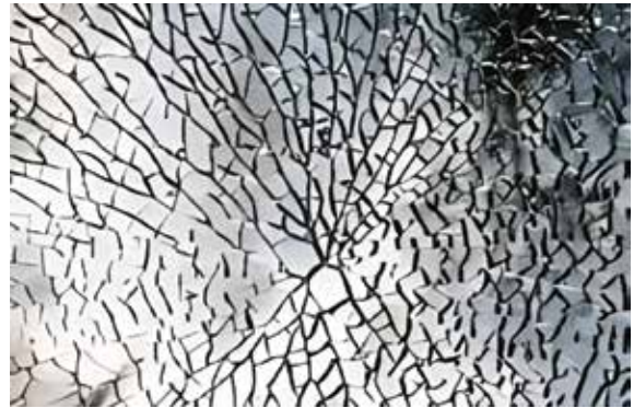
Fig. 1.1 “Starburst” and “butterfly” pattern spontaneous crack of fully tempered glass(1)
