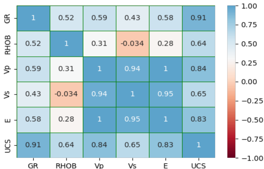
Figure 3: Heatmap of relationship between predictor and target variable of UCS.
