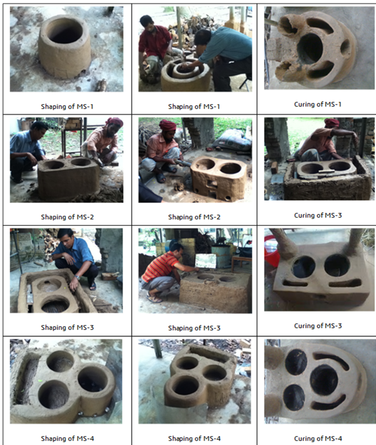
Figure 2: Mud-stove fabrication and curing processes
