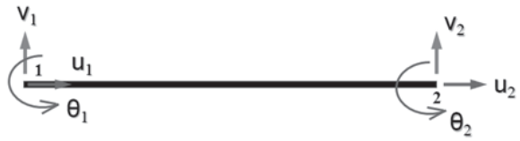
Fig.-1: 2D Beam Element with three degrees of freedom.
